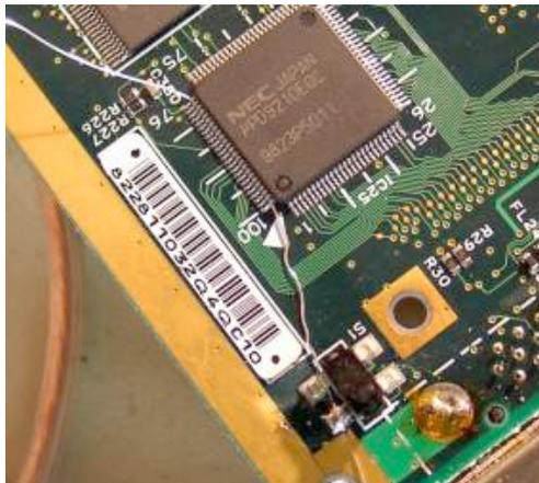
4. While gently pulling the wire out, go along heating each pad. The remaining solder should melt and the wire will slip under the pad. The wire will bend the pad up the slightest amount, which will prevent it from making contact with the solder again.
