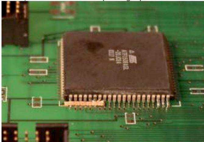
3. Take your soldering iron and heat the solder wick, which will heat the solder on the other side which will absorb into the solder wick
